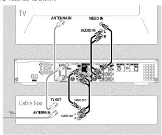
Connect the DVD-Recorder **directly** with your TV-set (Cable from the output jacks **S-VIDEO** (Y/C)-OUT2 or **VIDEO** (CVBS)-OUT2 directly to the TV set). If there is a video recorder or another device in between, there can be distortions in the TV pictures from the 'copy protection system'.
